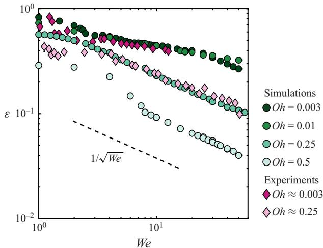
Figure 9. Variation of the restitution coefficient with the impact Weber number ( $We$ ) at different drop Ohnesorge numbers ( $Oh$ ). The simulations (circle data points) match perfectly with the experimental results (diamond data points) of Jha *et al.* (2020) without any fitting parameters. Here, the Bond number ( $Bo$ ) is 0.167.
