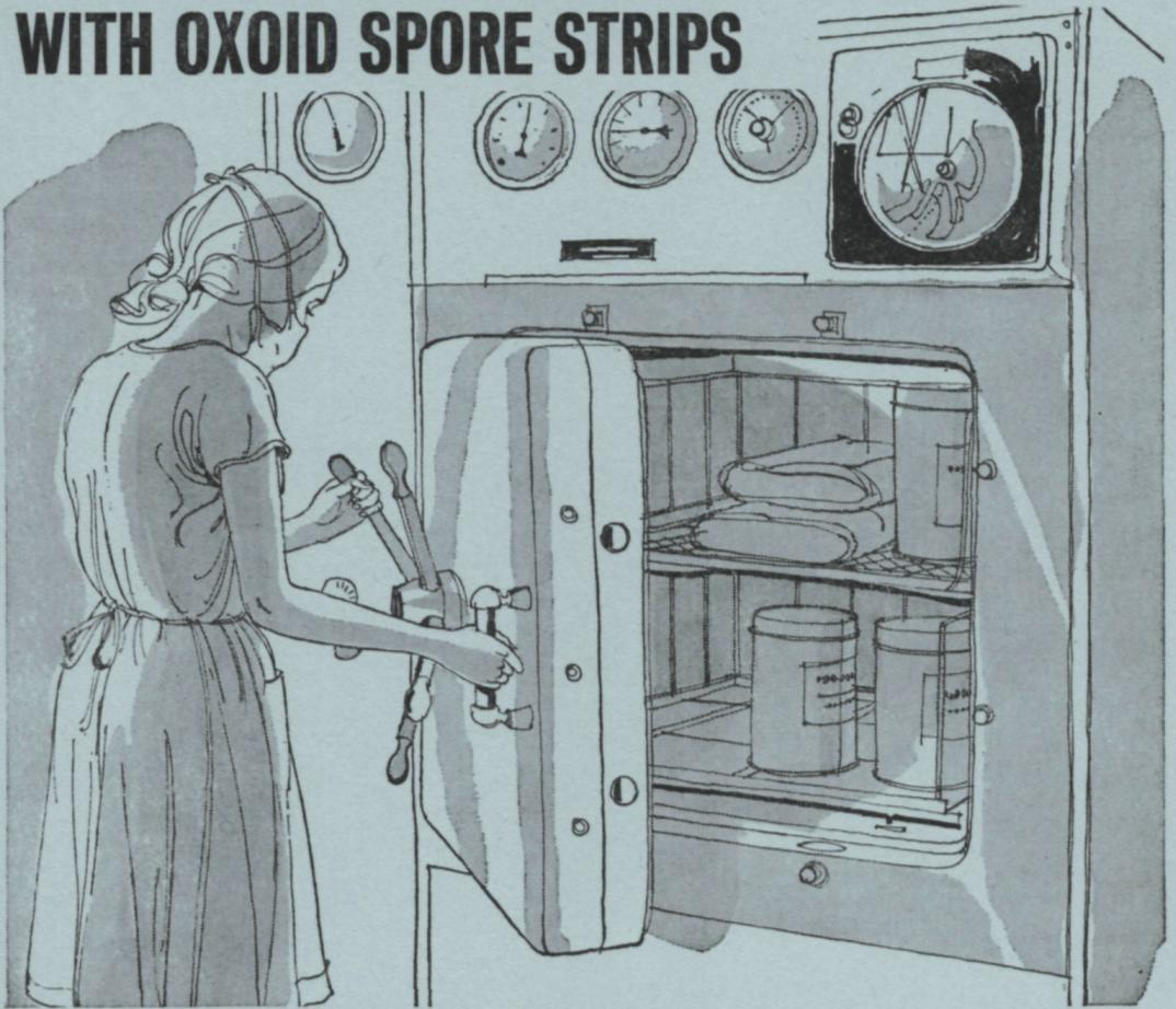
Oxoid Spore Strips give positive and dependable control of steam sterilization processes. They not only indicate that a temperature of 121°C. has been maintained for adequate time but they provide biological proof of sterilizing efficiency.
