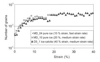
**Fig. 6.** Examples of grain number evaluation at different stages during the  $-7^{\circ}$ C deformation of the ice samples. These numbers account for volume changes during deformation with an error in the grain number determination of approximately  $\pm 400$  (see 'Methods' and 'Grain size evolution' sections for further descriptions).
