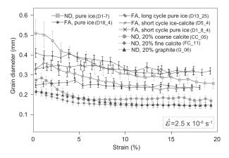
**Fig. 12.** The evolution of the average grain size of ice at small strain steps at strain rate  $2.5 \times 10^{-6} \, \mathrm{s}^{-1}$  (medium) obtained by neutron diffraction(ND) analysis and during in situ experiments on the fabric analyser (FA) and deformed at -7C. The average grain size is defined as a 3-D equivalent diameter. The error bars are between 15 and 20%.
