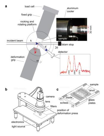
**Fig. 1.** Schematic illustrations showing the deformation set-up in the 3-D and 2-D experiments. (a) The Kowari instrument configuration for 3-D neutron diffraction and CPO analysis. Insets show deformed ice sample, from an initial sample that had a diameter ~2.5 cm, length ~3.2–4.0 cm and ice diffraction pattern. (b) Sketch of G50 fabric analyser. (c) Sketch of 2-D deformation press with outer covers and upper halves of anvils removed for clarity.
