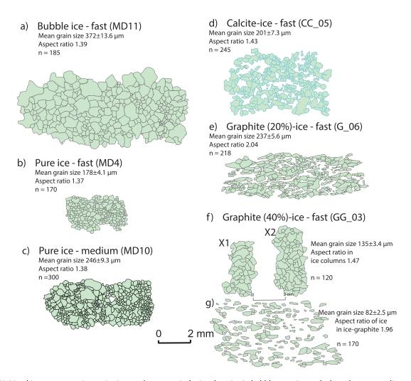
**Fig. 10.** Digitized images comparing grain sizes and aspect ratio for ice domains in bubble, pure ice and where there was a dispersed second phase. The background in (d) is fine calcite with grain size  $<150 \, \mu m$ . The background in (e) and (g) is graphite. n = number of grains digitized using ArcGIS from fabric analyser images. Bar scale of 2 mm applies to all images.
