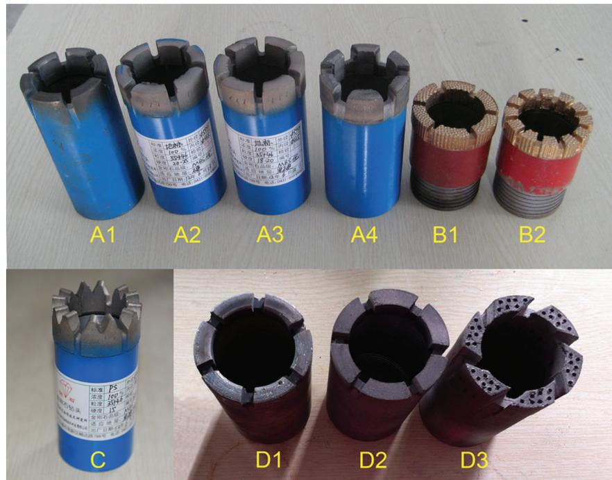
**Fig. 2.** Tested drill bits. A1–A4: impregnated bits; B1 and B2: surface-set bits; C: toothed impregnated bit; D1–D3: bionic impregnated bits.
