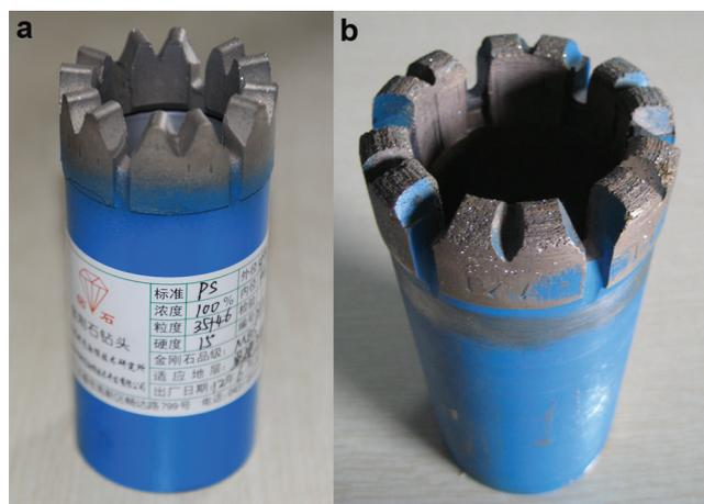
Fig. 7. New (a) and used (b) toothed drill bit C.
