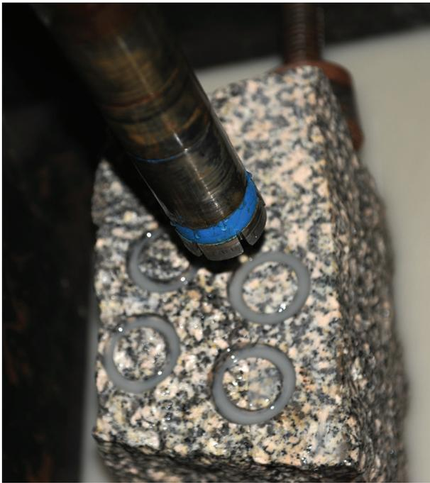
Fig. 4. Drill bit above the drilled borehole.
