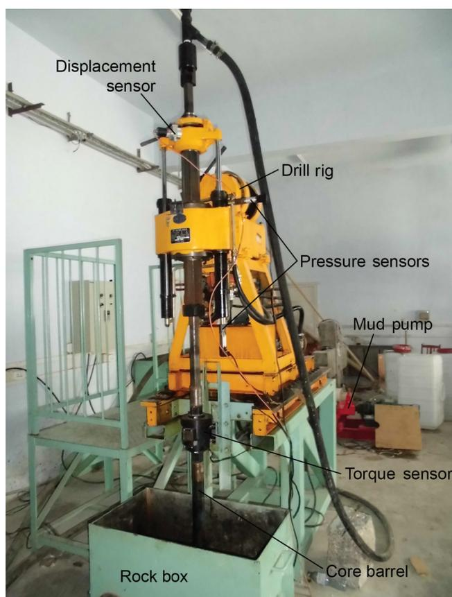
Fig. 1. Drill bit test stand.
