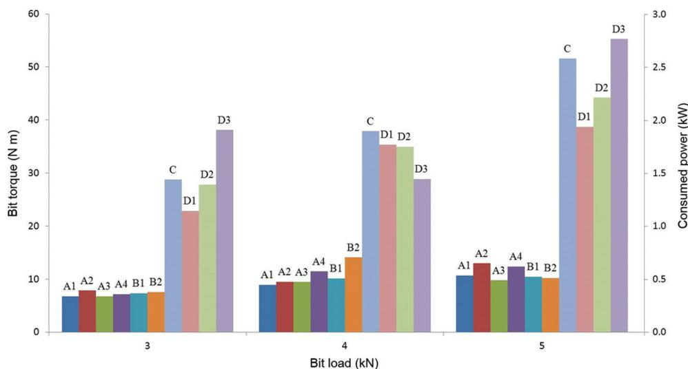
Fig. 6. Torque and consumed power vs bit load.
