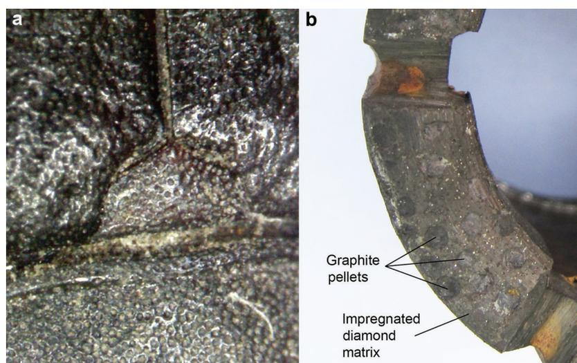
**Fig. 3.** (a) Armor surface of dung beetle ([http://www.f1cd.ru/media/reviews/ks-is\\_digilux/](http://www.f1cd.ru/media/reviews/ks-is_digilux/)). (b) Working face of bionic drill bit D1 type.
