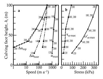
Fig. 5. Variation of velocity and stress indices with subaerial calving-face height,  $h_c$  (vertical axis). Points are labeled with values of total height at margin,  $h_0$ , commonly with two points being visually indistinguishable. (a) Speeds, including  $u_{\max}$ ,  $\Delta u_{\text{base}}$  and  $\Delta u_{\text{top}}$ . Values <1 m  $a^{-1}$  are omitted. (b) Maximum stresses, including  $\sigma'_{xx}$  and  $\tau_{xy}$ .
