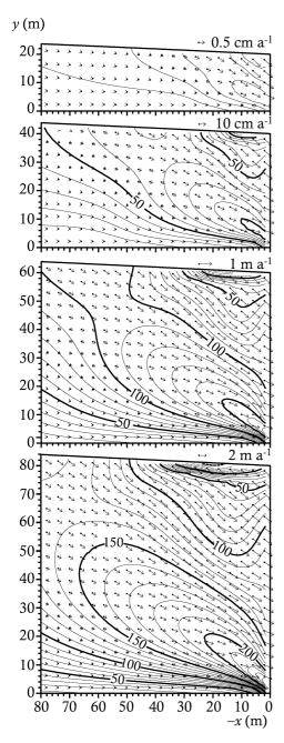
Fig. 7. Variation in  $\sigma'_{xx}$  (contours, 10 kPa interval) and velocity (vectors) for water-free, zero basal velocity simulations, where  $h_0(=h_c)$  varies from 20 m to 80 m in 20 m increments. Velocity vectors are shown at every other node for clarity. Scale of the velocity vectors varies dramatically with  $h_0$ : maxima given in Table 2 are scaled to a common length.
