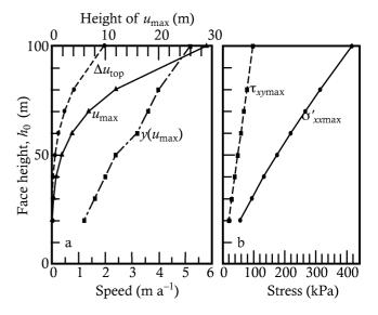
Fig. 6. Variation of velocity and stress indices with face height for water-free, zero basal velocity simulations listed in Table 2. (a) Speeds, including  $u_{\rm max}$  and  $\Delta u_{\rm top}$  along with the height at which  $u_{\rm max}$  occurs on the face, read against the upper axis. (b) Maximum values of  $\sigma'_{xx}$  and  $\tau_{xy}$  in the flowplane.
