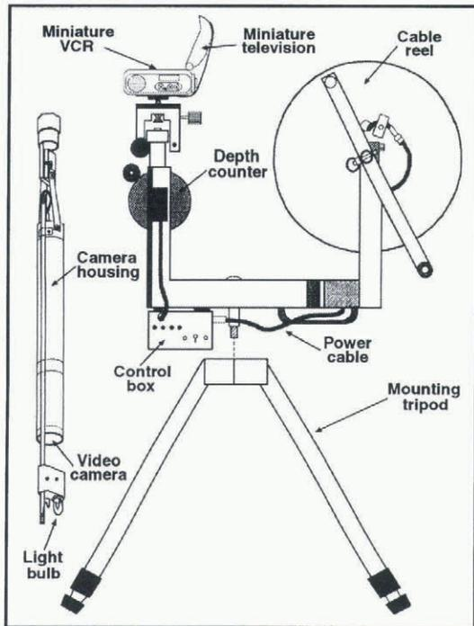
Fig. 3. The GeoVision Micro<sup>™</sup> borehole video-camera system (reproduced with permission from Marks Products, Inc.).
