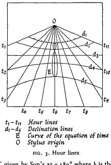
$h = l \sin \varphi \cot h$  and in a direction CT given by Sun's  $az \pm 180^{\circ}$  where h is the altitude and Z the azimuth of the Sun.
