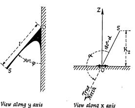
correct positioning of the FIG. 8. Positioning of the stylus for a vertical sundial
