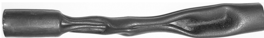
Figure 1.1. A copper tube suffering the effects of a lightning strike (Credit: Brian James, School of Physics, University of Sydney).
