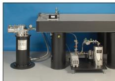
Existing liquid-helium-cooled microscopy cryostats can be converted to cryogen-free operation with the addition of an external cryocooler, the Janis Recirculating Gas Cryocooler (RGC4). Instead of using liquid helium from a storage vessel, the RGC4 delivers a stream of 4°K helium to the microscopy cryostat. This combination provides positional stability to <10 nm and is suitable for micro-PL, micro-Raman, and other vibration-sensitive techniques.
