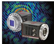
Princeton Instruments announced the SOPHIA-XO camera platform, specially designed for scientific applications such as VUV/EUV/XUV imaging, X-ray diffraction, X-ray microscopy, X-ray holography, X-ray spectroscopy, and X-ray plasma. The new SOPHIA-XO cameras use back-illuminated CCDs for direct detection of the widest range of VUV and X-rays (~5 eV to 30 keV). These new XO camera models are extensions of Princeton Instruments' popular SOPHIA® product line.
