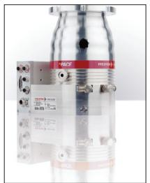
The Pfeiffer Vacuum HiPace M high-performance magnetically levitated turbopumps have high pumping speeds (300 l/s, 700 l/s, and 800 l/s), have high gas throughput, and achieve high compression ratios for all gases. These pumps are optimized to run in all mounting orientations with a low vibration signature and quiet operation. An advanced rotor design provides unlimited rotor service life, out of balance compensation, and dependable operation. They are maintenance-free and oil-free.
