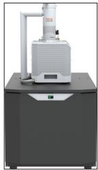
The newly released Thermo Scientific Prisma SEM platform incorporates an extensive selection of detectors, *in situ* stages, automation packages, and its environmental mode to make it one of the most complete offerings on the market. It can be configured as a lean “point-and-shoot” solution for industrial customers or augmented with an array of specialized imaging and analysis options for the researcher. It lets customers buy confidently, knowing they have an optimal solution for their needs.
