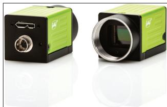
JAI has added a new model to its Go Series of small and versatile machine vision cameras. The GO-5100MP-USB is built around Sony’s IMX250MZR polarized CMOS image sensor, offering 5.1 megapixels of total resolution and an innovative 4-way polarized filter design creating a range of possibilities for imaging and analysis of objects. The camera features a full resolution of 2464 × 2056 pixels with a 2/3" optical format and pixel sizes of 3.45 µm × 3.45 µm.
