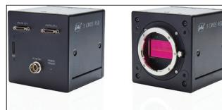
JAI has introduced a new 3-CMOS prism color line scan camera in its Sweep+ Series camera family. The new SW-4000T-MCL features three custom CMOS line sensors with 4K resolution mounted on a high-grade optical prism assembly that precisely splits the incoming light into red, green, and blue wavebands. The new camera provides 24-bit non-interpolated RGB output at up to 67.7 kHz, more than four times faster than any previous 4K prism color line scan camera.
