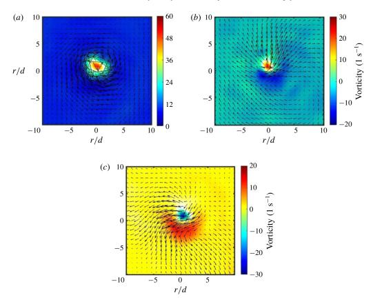
FIGURE 10. (Colour online) Velocity vectors and vorticity field of (a) first, (b) second and (c) third POD mode for a jet with  $Re_0 = 2300$ , at  $\Omega = 0.21$  rad s<sup>-1</sup>, for z/d = 0.5.
