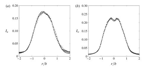
FIGURE 3. Non-dimensionalized r.m.s. values of the (a) radial  $I_u$  and (b) vertical  $I_w$  velocity components as a function of the non-dimensional distance r/b from the centre of the jet for  $5 \le z/d \le 25$ .
