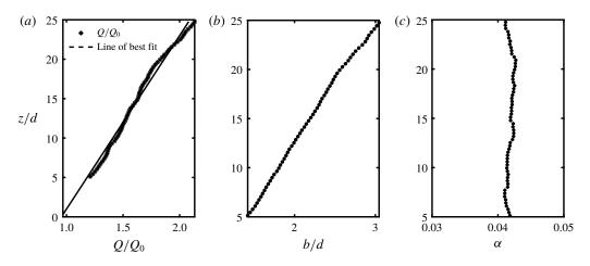
FIGURE 5. Variation of (a) non-dimensionalized vertical, volumetric flow rate,  $Q(z)/Q_0$ ; (b) non-dimensional plume radius, b/d; (c) entrainment coefficient  $\alpha(z)$  with vertical height z/d above the source.
