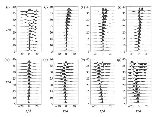
FIGURE 9 (cntd). Instantaneous vector fields of the vertical velocity component w(r) for a jet with  $Re_0 = 2300$  at  $\Omega = 0.21$  rad s<sup>-1</sup> at times t of (a) 6 s, (b) 10 s, (c) 14 s, (d) 18 s, (e) 22 s, (f) 26 s, (g) 30 s, (h) 34 s, (i) 38 s, (j) 42 s, (k) 46 s, (l) 50 s, (m) 54 s, (n) 58 s, (o) 62 s and (p) 66 s.
