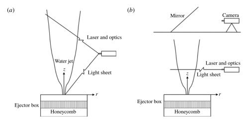
FIGURE 1. Illustration of ejector box and set-up for PIV measurements in the (a) vertical z-r plane and (b) horizontal  $\theta$ -r plane. A technical drawing illustrating the scale of Warwick's large rotating-tank facility, inside which the ejector box is positioned, is displayed as figure S1 in the supplementary material available at https://doi.org/10.1017/jfm.2019.186.
