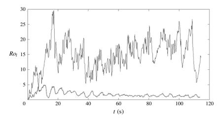
FIGURE 22. Variation of  $Ro_l$  with time, near the source at z/d = 0.5, for a jet with  $Re_0 = 16\,000: \dots, Ro_0 = 653, \ \Omega = 0.42 \text{ rad s}^{-1}; \dots, Ro_0 = 1055, \ \Omega = 0.73 \text{ rad s}^{-1}.$
