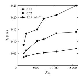
FIGURE 14. Variation of formation-breakdown frequency,  $f_{\theta}$ , of the jets as a function of the Reynolds number  $Re_0$  at  $f_T = 0.033$  ( $\Omega = 0.21$  rad s<sup>-1</sup>).
