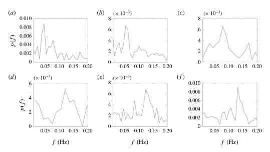
FIGURE 18. Fourier spectra for the temporal variation of the kinetic energy associated with azimuthal velocity components,  $Re_0 = 2300$ , for six different rotation rates, in units rad s<sup>-1</sup>: (a) 0.21, (b) 0.31, (c) 0.42, (d) 0.84, (e) 0.94 and (f) 1.05.
