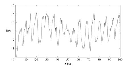
FIGURE 20. Variation of the instantaneous, local Rossby number,  $Ro_l$ , with time, for a jet with  $Re_0 = 2300$  at  $\Omega = 1.05$  rad s<sup>-1</sup>, corresponding to  $Ro_0 = 60$ , near source at z/d = 0.5.
