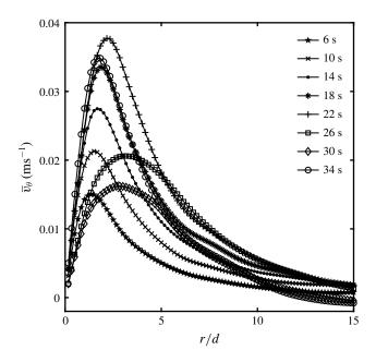
FIGURE 16. Profiles of the circumferentially averaged azimuthal velocity component  $\overline{v}_{\theta}$  as a function of the distance r/d from the centre for different instants in time.
