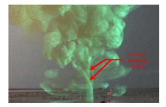
FIGURE 7. (Colour online) Fluorescein visualization of the stem of a jet revealing the two cyclonically upward-spiralling helical strands for  $Re_0 = 2300$  at  $\Omega = 0.21$  rad s<sup>-1</sup>. A supplementary movie is available at https://doi.org/10.1017/jfm.2019.186.
