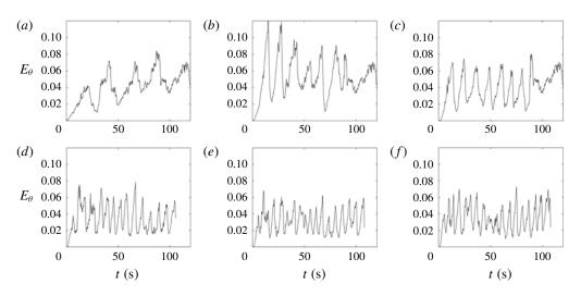
FIGURE 17. Temporal variation of the kinetic energy associated with azimuthal velocity component, at  $Re_0 = 2300$ , for six different rotation rates, in units rad s<sup>-1</sup>: (a) 0.21, (b) 0.31, (c) 0.42, (d) 0.84, (e) 0.94 and (f) 1.05.
