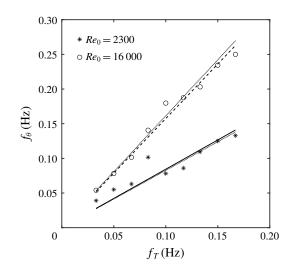
FIGURE 19. Formation-breakdown frequency,  $f_{\theta}$ , of the jets as a function of the background rotation frequency,  $f_T = \Omega/2\pi$ , of the turntable: \*, —,  $Re_0 = 2300$ ,  $f_{\theta} = 0.84f_T$ ; O, ---,  $Re_0 = 16\,000$ ,  $f_{\theta} = 1.57f_T$ . The dotted lines in the immediate vicinity of the two least-squares interpolations are the corresponding data interpolations from figure 13 obtained in § 4.3.1 from the POD analysis.
