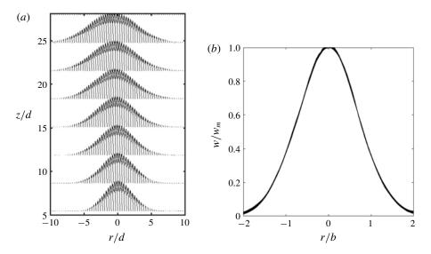
FIGURE 2. (a) Time-averaged velocity profiles at eight different heights z/d as a function of r/d; (b) collapsed datasets after fitting Gaussian profiles and non-dimensionalizing accordingly for  $5 \le z/d \le 25$ .
