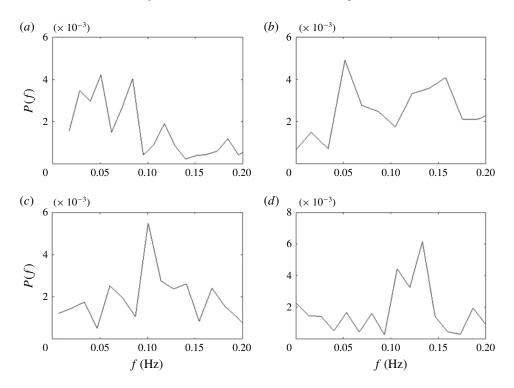
FIGURE 12. (Colour online) Fourier spectra for the time coefficient,  $c_1(t)$ , of the first POD mode for a jet with  $Re_0 = 2300$  for four different rotation rates: (a)  $\Omega = 0.21$  rad s<sup>-1</sup>, (b)  $\Omega = 0.41$  rad s<sup>-1</sup>, (c)  $\Omega = 0.73$  rad s<sup>-1</sup> and (d)  $\Omega = 1.05$  rad s<sup>-1</sup>.
