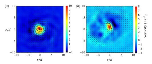
FIGURE 15. (Colour online) Two examples illustrating the performance of the centrefinding process of Graftieaux *et al.* (2001) applied to flow fields from the current experiments for  $Re_0 = 2300$ , at  $\Omega = 0.21$  rad s<sup>-1</sup>, with (a)  $\Gamma = 0.87$  and (b)  $\Gamma = 0.66$ . Centres are identified in both plots through a bold black cross.
