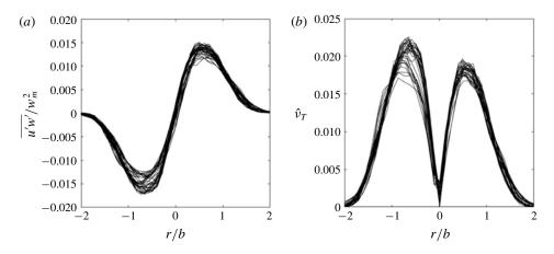
FIGURE 4. Non-dimensionalized (a) Reynolds stress and (b) turbulent viscosity as a function of the non-dimensional distance r/b from the centre of the jet for  $5 \le z/d \le 25$ .
