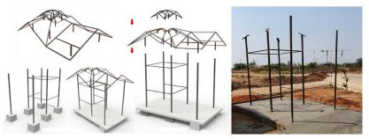
Figure 5: Frame structure for prototyping
