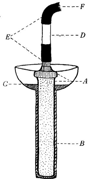
Fig. 1. A = coating of collodion; B = special glass container; C = highest level of filtering liquid; D = glass connecting tube; E = rubber tubing; F = connexion to negative pressure.
