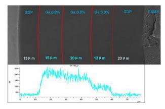
**Figure 3.** Cross-sectional SEM image and EDS results of GPD shell graded doped with Ge.
