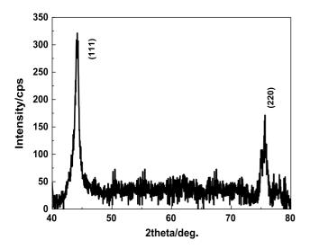
Figure 9. XRD pattern of HDC shell.
