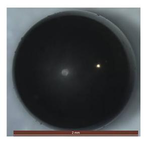
Figure 8. Microphotograph of HDC shell.
