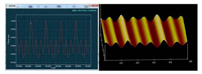
Figure 10. Designed locus for the diamond cutter and AFM image of the modulating sample surface.
