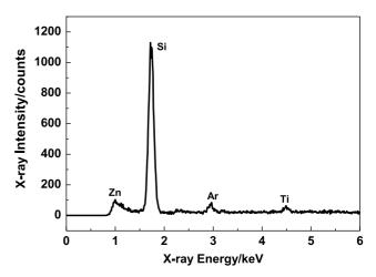
Figure 6. XRF spectrum of an argon filled Si:GDP.
