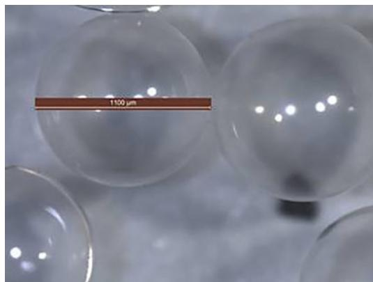
**Figure 5.** Photograph of HGM made by Si:GDP method.
