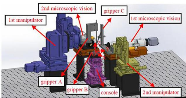
**Figure 12.** Configuration of the semi-automatic assembly system.
