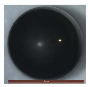
Figure 8. Microphotograph of HDC shell.
