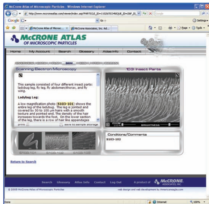
Figure 2. Particle Characterization Viewer: The viewer features analysis tabs located across the top of the viewer, a particle description window on the left with the image thumbnail scroll viewing viewer below, and the image window on the right with the image detail window below it.
