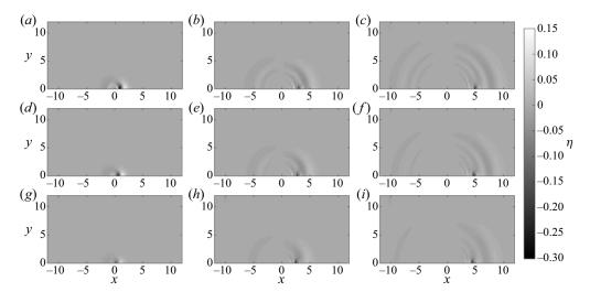
Figure 19. The free surface elevations generated by an initially stationary Gaussian-shaped bottom obstacle  $(\epsilon = 0.3, \mu = 0.3)$  accelerating for a duration of  $t_{acc}$  until it reaches the normalised constant speed Fr = 0.5. The results are numerically simulated based on WNWD. (a-c) Instantaneous acceleration,  $t_{acc} \rightarrow 0$ ; (d-f)  $t_{acc} = 1$ ; (g-i)  $t_{acc} = 2$ . For (a,d,g) t = 2; (b,e,h) t = 6; (c,f,i) t = 10.
