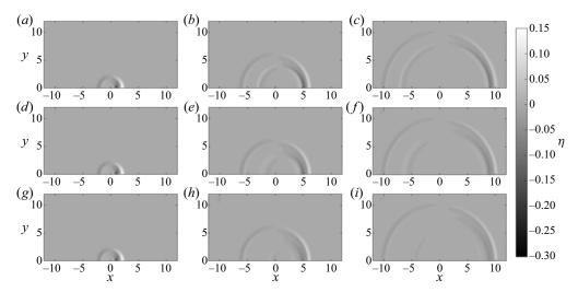
Figure 20. The free surface elevations generated by a Gaussian-shaped bottom obstacle which suddenly starts moving at a normalised constant speed Fr = 0.5 for a duration of  $t_{Fr} = t_{sep}(0) = 2$ , before decelerating to a halt over a duration of  $t_{dec}$ . The results are numerically simulated based on LSWE. (a-c) Instantaneous deceleration,  $t_{dec} \rightarrow 0$ ; (d-f)  $t_{dec} = 1$ ; (g-i)  $t_{dec} = 2$ . For (a,d,g) t = 2; (b,e,h) t = 6; (c,f,i) t = 10.
