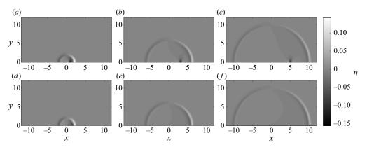
Figure 8. The free surface elevations predicted by the linear shallow water analytical solutions at three different times, with Fr = 0.5 and the Gaussian-shaped  $B_0$  given in (2.28). (a-c) The complete integral-form solution (2.18) in the shallow water limit,  $\mu \to 0$ ; (d-f) the far-field solution (2.32), accurate for large r for (a,d) t = 2; (b,e) t = 6; (c,f) t = 10.
