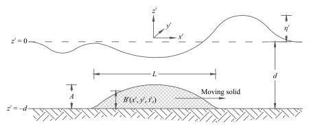
Figure 1. A dimensional definition sketch of water waves generated by a moving bottom obstacle. Both the free surface displacement and the thickness of the obstacle are assumed small in linear wave models; such assumptions are not needed in nonlinear wave models. This study considers only bottom obstacles translating at a subcritical speed.
