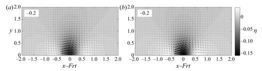
Figure 10. The wave and velocity fields (at the still water surface z=0) associated with the 'trapped wave' analytical solutions, with Fr=0.5,  $\mu=0.3$  and the Gaussian-shaped  $B_0$  given in (2.28). (a) The integral-form solutions (2.18), shown in the supplementary material, for the trapped wave only; (b) the integral-form solutions in the shallow water limit,  $\mu \to 0$ .
