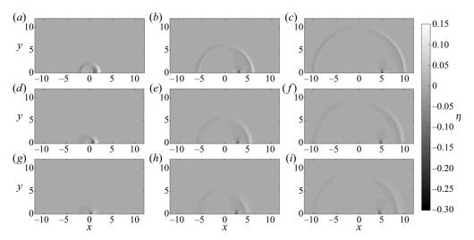
Figure 16. The free surface elevations generated by an initially stationary Gaussian-shaped bottom obstacle accelerating for a duration of  $t_{acc}$  until it reaches the normalised constant speed Fr = 0.5. The results are numerically simulated based on LSWE. (a-c) Instantaneous acceleration,  $t_{acc} \rightarrow 0$ ; (d-f)  $t_{acc} = 1$ ; (g-i)  $t_{acc} = 2$ . (a,d,g) t = 2; (b,e,h) t = 6; (c,f,i) t = 10.
