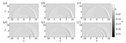
Figure 12. The free surface elevations predicted by different wave models at t = 10, with Fr = 0.5,  $\epsilon = 0.3$ ,  $\mu = 0.3$  and the Gaussian-shaped  $B_0$  given in (2.28). (a) LSWE; (b) NSWE; (c) the far-field shallow water solution (2.32), accurate for large r; (d) LWD; (e) WNWD; (f) the first term of the far-field leading wave solution (2.22), accurate for large r and near r = t.
