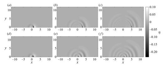
Figure 4. The free surface elevations predicted by the linear and fully dispersive analytical solutions at three different times, with Fr = 0.5,  $\mu = 0.3$  and the Gaussian-shaped  $B_0$  given in (2.28). (a-c) The complete integral-form solution (2.18); (d-f) the first term of the far-field leading wave solution (2.22), accurate for large r and near r = t for (a,d) t = 2; (b,e) t = 6; (c,f) t = 10.
