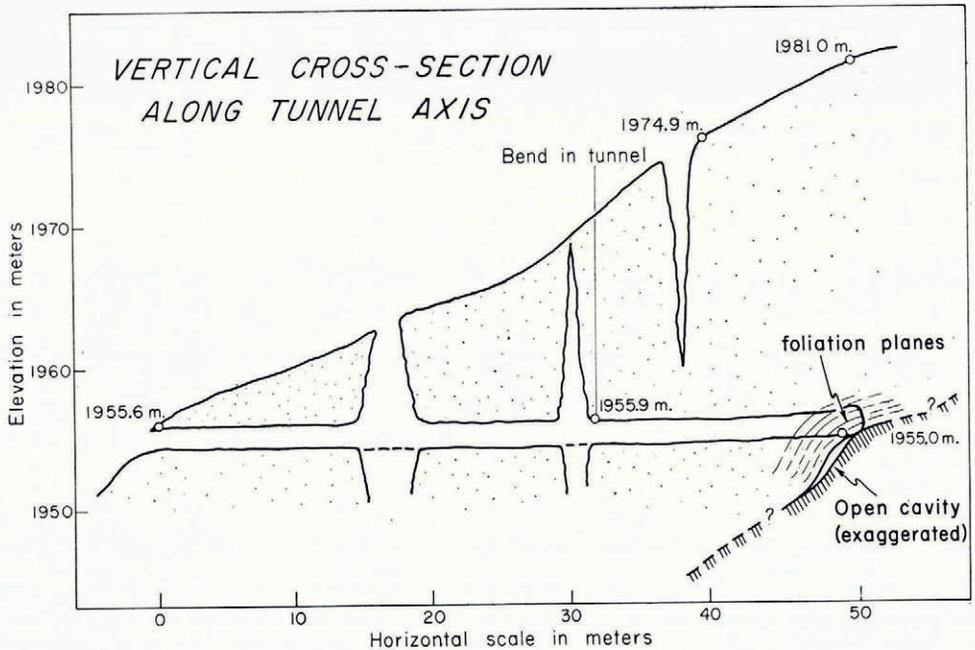
Fig. 2. Vertical cross-section along axis of tunnel. Configuration of ice foliation near the tunnel head is indicated, and ice separation from bedrock is shown schematically. Crevasses shown approximately only
