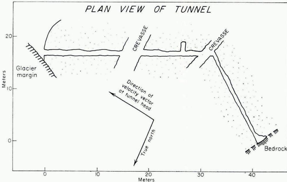
Fig. 1. Plan view of tunnel in Blue Glacier, excavated June–July 1962. Observations reported were made in chamber at head of tunnel, adjacent to bedrock
