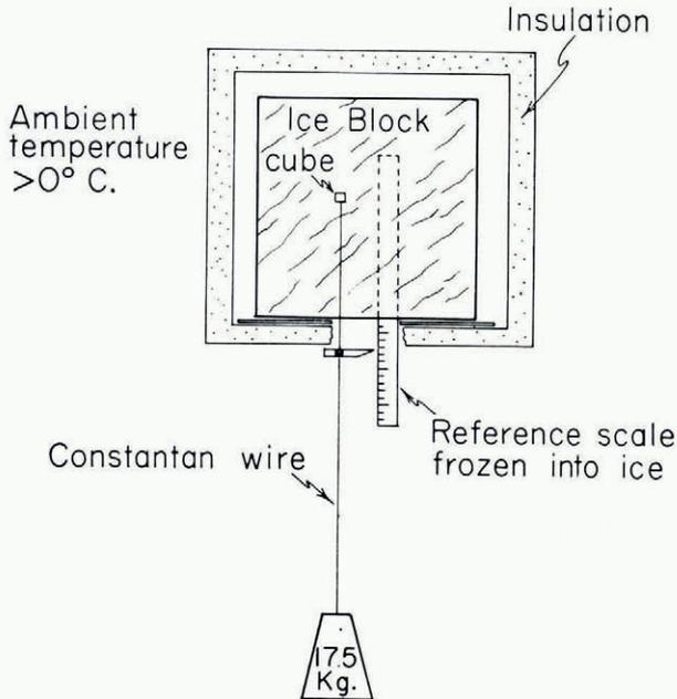
Fig. 8. Arrangement for experimental study of regelation flow
