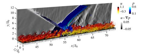
FIGURE 4. (Colour online) STBLI base flow: instantaneous isosurfaces of the Q-criterion coloured by streamwise velocity highlight hairpin vortices. The shocks (in blue) and background shading are indicated by an isosurface and contours of  $u \cdot \nabla p$ .
