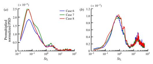
FIGURE 12. (Colour online) Wall pressure perturbation power spectral densities demonstrating the linearity of forcing and attenuation for cases 6–8. The PSDs have been normalized by  $(\Phi_{\alpha}^{P_{Ltarget}})^2$  to demonstrate collapse of the spectra. (*a*) Wall pressure perturbation power spectral density at the time-mean separation point. (*b*) Wall pressure perturbation power spectral density downstream of the reattachment point ( $x^* = 1.1$ ).
