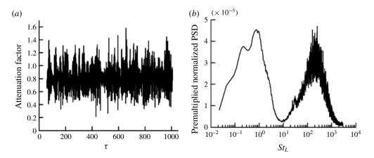
FIGURE 13. Discrete variable attenuation-factor signal and power spectral density for the self-sustaining perturbations of case 11. (a) Discrete variable attenuation-factor signal:  $1 - \alpha \Delta \tau$ . (b) Pre-multiplied and normalized power spectral density of discrete variable attenuation factor.
