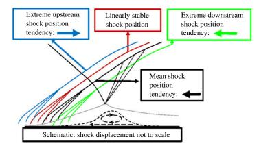
FIGURE 15. (Colour online) Schematic indicating the linear restoring tendencies of the reflected shock at extreme upstream (phase  $\pi/2$ ) and downstream (phase  $3\pi/2$ ) displacements. The 'time-mean shock position' (which has a linear tendency for upstream motion) does not coincide with the 'time-mean linearly stable shock position' as first indicated in figure 8.
