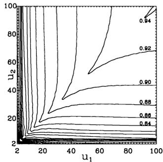
Fig. 2. Visibility Loss Contours of a range of optical coordinates,  $u_1$  and  $u_2$ , in the two arms of a stellar interferometer. The contours represent visibility loss calculated for the geometrical beam.
