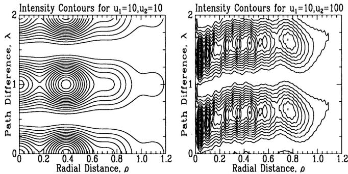
Fig. 1. Fringe distortion due to diffraction effects for two combinations of  $u_1$  and  $u_2$ . Here,  $u_1$  and  $u_2$  are propagation variables with the form  $u = ka^2/z$ , where  $k$  is wave number,  $a$  is aperture radius, and  $z$  is the propagation distance from the siderostat.
