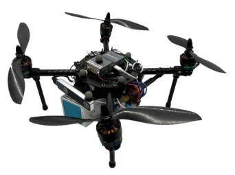
*Figure 16.* UAV used for flight tests. The payload consists of an Intel NUC, a Livox MID-70, and an Intel Realsense T265.
