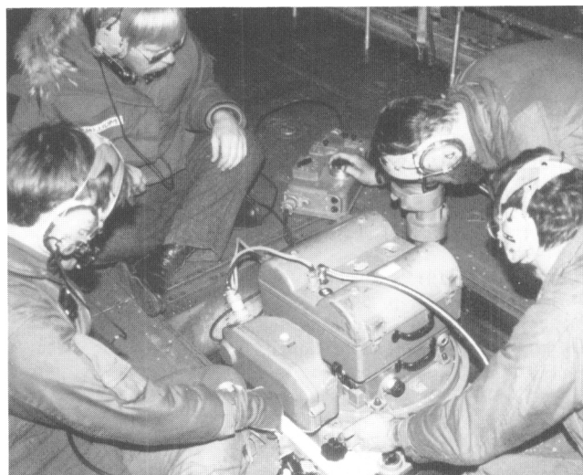
Fig. 1. RC-8 mapping camera mounted in U.S. NSF/Navy C-130 aircraft. Recently used by U.S. Geological Survey for aerial photography of ice streams and crevasse fields in West Antarctica (Vornberger and Whillans, 1986).
