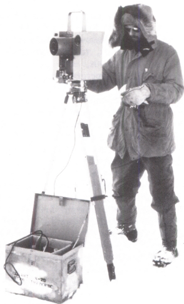
Fig. 12. Electronic distance-measuring device in Antarctica around 1980 (unknown source).
