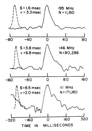
Fig. 3. Average pulse profiles of JP 1933 at low radio frequencies (solid lines). The dotted profile is that profile which would be observed if the pulse profile were independent of frequency. The IF bandwidth of 10 kHz caused a dispersion smearing of S, the post detection RC time constant was  $\tau$ , and the number of pulses averaged was N. The zero corresponds to the zero time phase when the delay due to dispersion,  $\int n_e dl = 158.60 \pm 0.05 \text{ pc cm}^{-3}$ , is corrected for.
