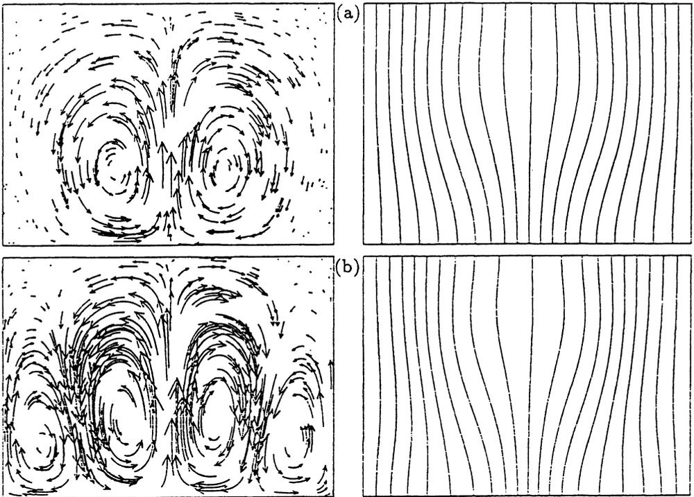
Figure 1. Nonlinear convection in a stratified compressible layer ( $0.2 \leq \zeta \leq 2.2$ ). Streaklines (left) and fieldlines (right) for steady solutions with (a)  $R = 1.07 R_0$  and (b)  $R = 1.39 R_0$ . Note the development of countercells in the corners.
