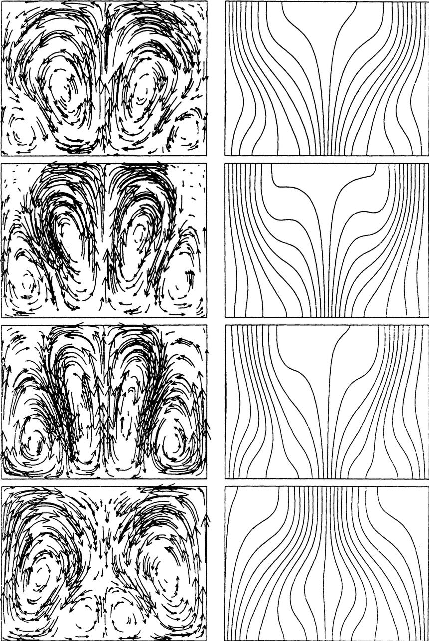
Figure 2. Oscillatory convection in a stratified layer for  $R = 2.59 R_0$ . Streaklines and fieldlines at successive intervals during half a period of the oscillation.
