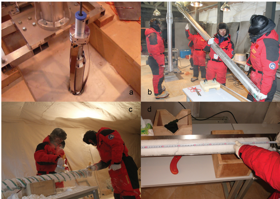
Fig. 9. Working events during the first drilling season at Kunlun station: (a) lowering shallow drill; (b) lifting the drill; (c) cleaning the drill and removing the core; and (d) core processing.
