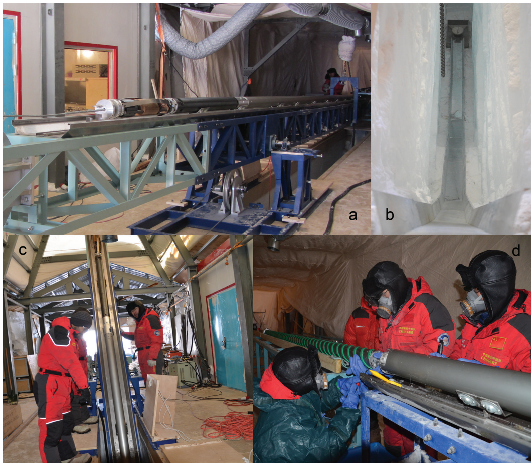
Fig. 15. Working events during the second drilling season at Kunlun station: (a) drill rig assembly; (b) fluid back-flow slot installation; (c) lowering the drill; and (d) cleaning the drill and removing the core.
