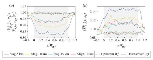
**Figure 14.** (a) Horizontal inflow velocity and (b) turbulence intensity at hub height. The average is taken from x = 10D to 2D in front of each wind farm. The shaded area represent the wind farm position.
