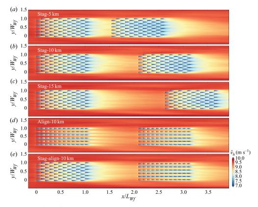
*Figure 4.* Time-averaged horizontal velocity magnitude at hub height.
