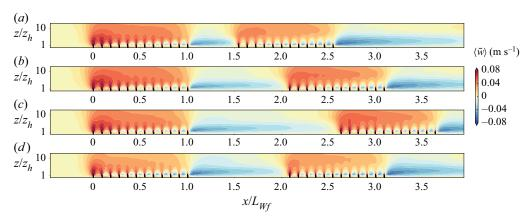
**Figure 8.** The vertical velocity, averaged over time and the spanwise wind farm extent for cases (a) stag-5 km, (b) stag-10 km, (c) stag-15 km and (d) align-10 km. The vertical extent is magnified by a factor of two to increase the visibility.
