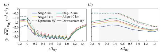
**Figure 13.** The vertical kinetic energy flux, averaged over time and the spanwise wind farm extent at (a) h = 160 m and (b) h = 400 m. The shaded area indicates the wind farm position.
