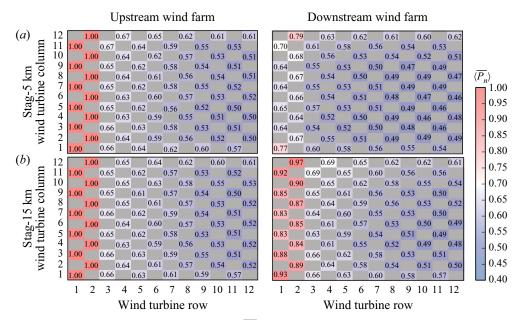
**Figure 18.** Map of turbine power production  $\langle \overline{P_n} \rangle$  for case (a) stag-5 km and (b) stag-15 km. All the entries have been normalized by the power of the turbines in the first or second row of the respective column.
