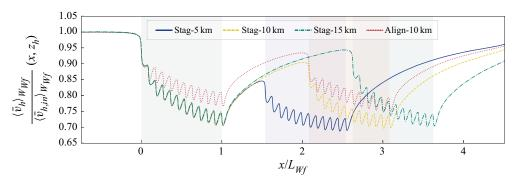
Figure 5. Horizontal velocity magnitude at hub height normalized by its inflow value averaged over the spanwise extent of the wind farm. The shaded regions indicate the streamwise location of each farm.
