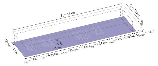
*Figure 1.* Schematic of the computational domain, showing the wind farm layout and the fringe layer configuration. The distance between the farms  $\Delta x_{Wf}$  is varied from 5 to 15 km.
