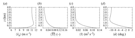
**Figure 2.** Temporally and horizontally averaged inflow conditions. (a) Horizontal velocity magnitude, (b) turbulence intensity, (c) vertical momentum flux and (d) wind angle as a function of height. The shaded area indicates the vertical extent of the wind turbines.
