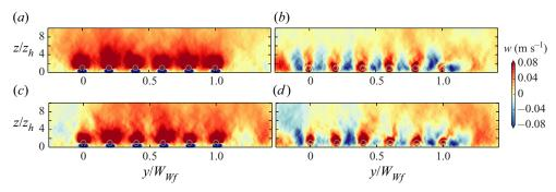
**Figure 7.** Time-averaged vertical velocity at the (a) first and (b) last row of the upstream wind farm, and the (c) first and (d) last row of the downstream wind farm for case align-10 km. Grey circles denote the wind turbine positions.
