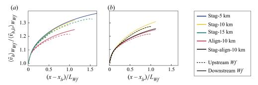
**Figure 16.** Horizontal velocity magnitude at hub height normalized with the velocity at 1.5D behind the last turbine row  $(x_{lr})$  and averaged over the spanwise extent of either (a) each wind farm or (b) the aligned wind farm.
