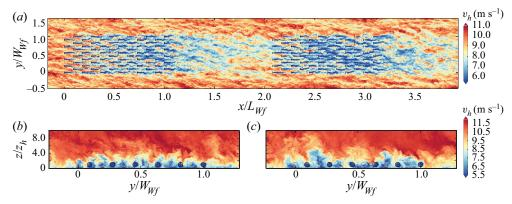
**Figure 3.** Instantaneous horizontal velocity magnitude  $v_h = \sqrt{u^2 + v^2}$  (a) at hub height, (b) 1D behind the last row of the upstream wind farm and (c) 1D behind the last row of the downstream farm. The positions of the wind turbines are marked by (a) black lines and (b,c) circles. Circles indicate the spanwise-vertical location of the turbines for uneven (grey) and even (black) turbine rows.
