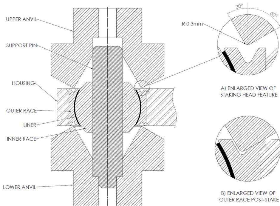
Figure 1. Cross-sectional schematic of the staking process
