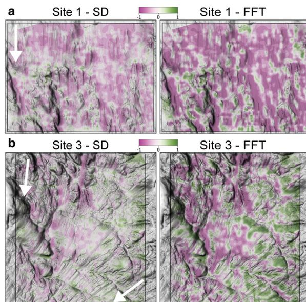
**Figure 6.** Anisotropy values calculated at every intersection point between parallel and orthogonal transects at sites 1 (a) and 3 (b) represent directionality of roughness measurements at the local scale. Orthogonal roughness dominates in the purple shades, parallel dominates in the green. White/gray shades indicate isotropic or random surfaces. White arrows indicate direction of paleo-ice flow.
