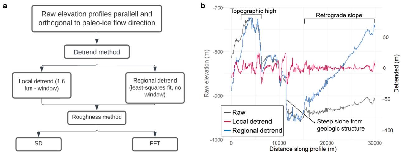
**Figure 3.** (a) Flow chart outlining the steps taken to calculate roughness using the SD and FFT methods described in the Methods section. (b) Example of a single raw elevation profile and corresponding detrended profiles using a local (red) and regional (blue) detrend method. Profile comes from Figure 2a.
