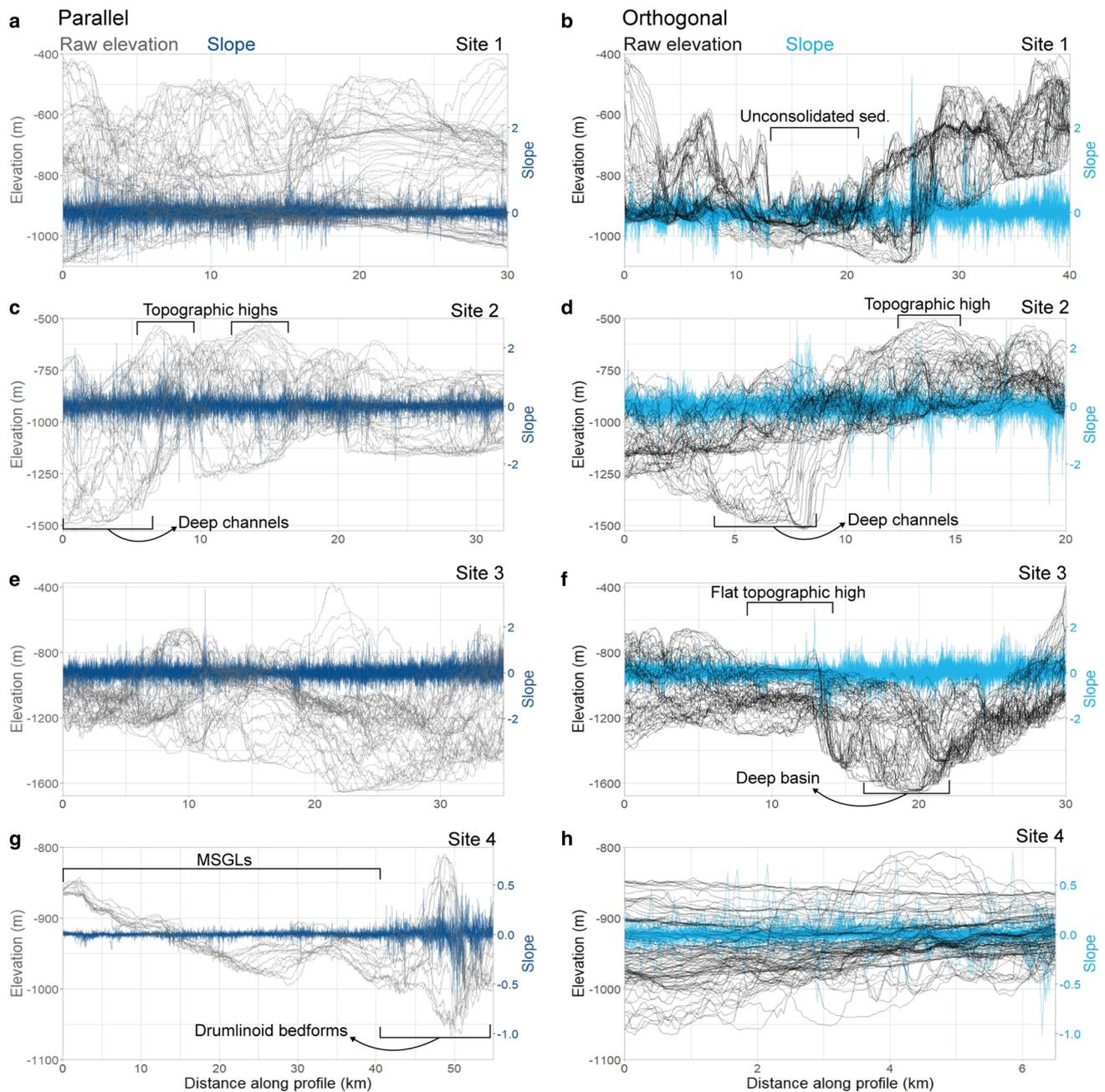
**Figure 2.** Raw elevation transects and calculated slope transects, both of which have data points at 50 m increments for East Amundsen Sea sites. Left and right columns show transects in the parallel and orthogonal orientations relative to paleo-ice flow direction, respectively. Slope is calculated as the dimensionless ratio of the vertical to horizontal change at every 50 m increment.
