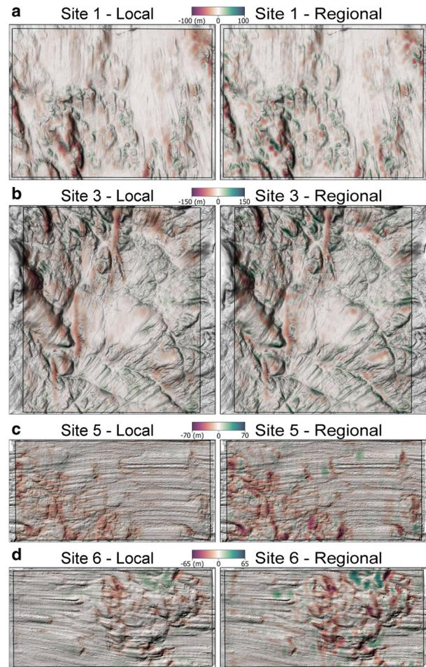
**Figure 7.** Difference in roughness measurements of parallel transects between high-resolution topography and BedMachine, showing where BedMachine under- and over-estimates roughness (red and green shades, respectively). Roughness for sites 1 and 3 (a, b) is derived from bathymetry; sites 5 and 6 (c, d) is from swath-radar (Holschuh and others, 2020).
