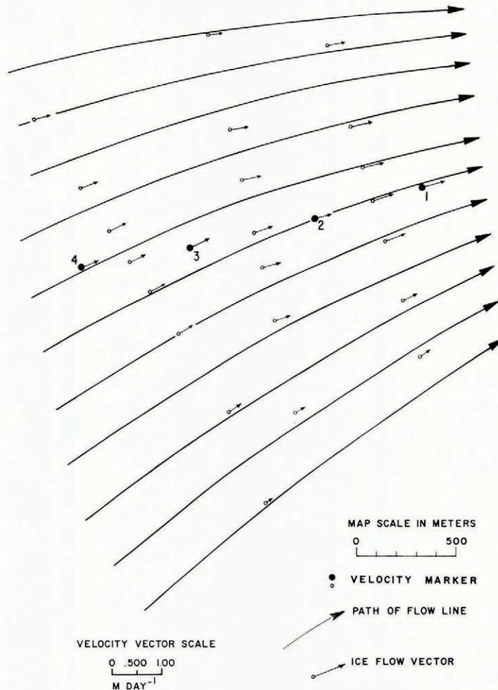
Fig. 4. Configuration of flow-line field based on velocity data, Kaskawulsh Glacier.
