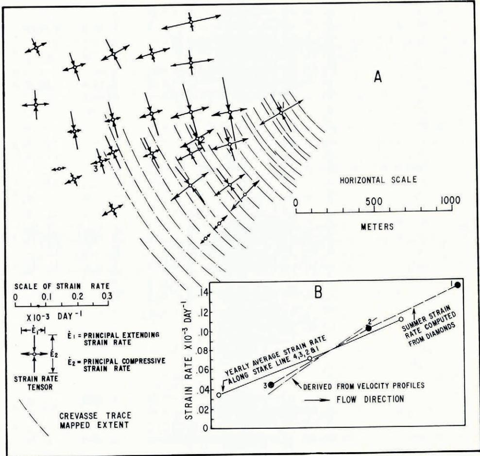
Fig. 8. (a) Configuration of principal strain-rate field in region of the transverse crevasses. (b) Longitudinal variation of principal extending strain-rate.
