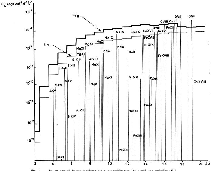
FIG. 1. — The energy of bremsstrahlung  $(E_{ff})$ , recombination  $(E_{fg})$  and line emission  $(E_L)$  in the region of the spectrum 2-20 Å for  $Te = 2.10^6 \text{ oK}$ .
