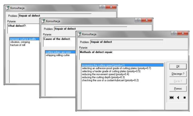
Fig. 8. Elimination of defects in milling operations.
