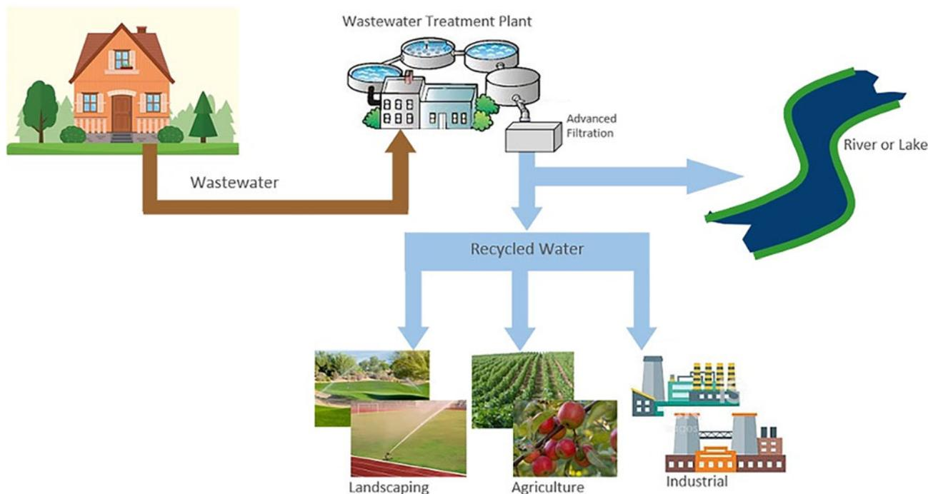
**Fig. 1.** Illustration showing the process whereby a wastewater treatment plant equipped with advanced filtration turns wastewater into municipal recycled water (figure presented in Section 3 of the survey).
