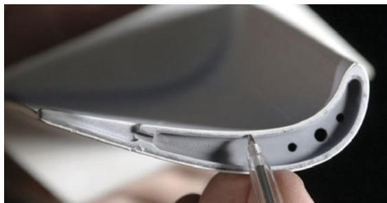
Figure 2. The 300- $\mu\text{m}$ -thick coating developed by Werner Stamm at Siemens to increase the service life and temperature resistance of turbine blades. Image provided by Siemens AG.
