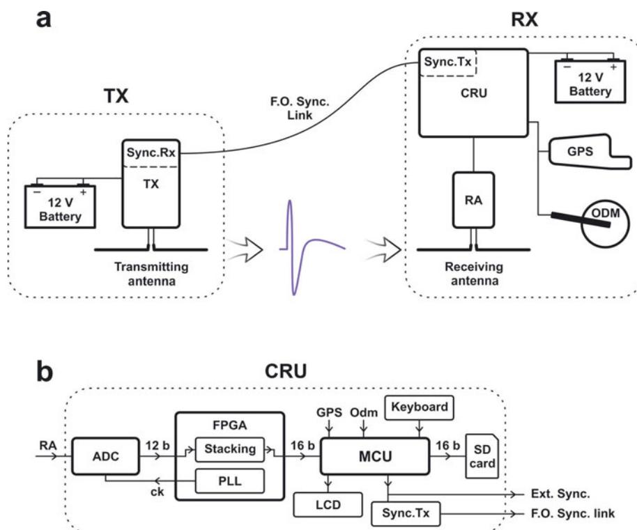
**Fig. 1.** (a) The TX is connected to a power supply (12.6 V) and the transmitting antenna and receives a synchronization signal from the RX. The RX (CRU + RA) controls the system and is connected to the receiving antenna, a power supply (12.6 V), a GPS receiver and a possible odometer, and transmits the synchronization signal to the TX. (b) The analog signal from the RA received at the CRU is 12-bit digitized, stacked and recorded using 16 bit per sample (four zero bits added) on the SD card.
