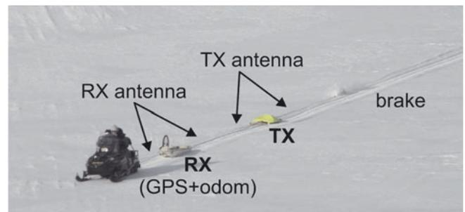
**Fig. 4.** Profiling during spring 2010 field tests in Svalbard using the 20 MHz antennas. A single scooter is leading the convoy, with the RX and TX placed on separate small sledges. An odometer is placed on the leading sledge.
