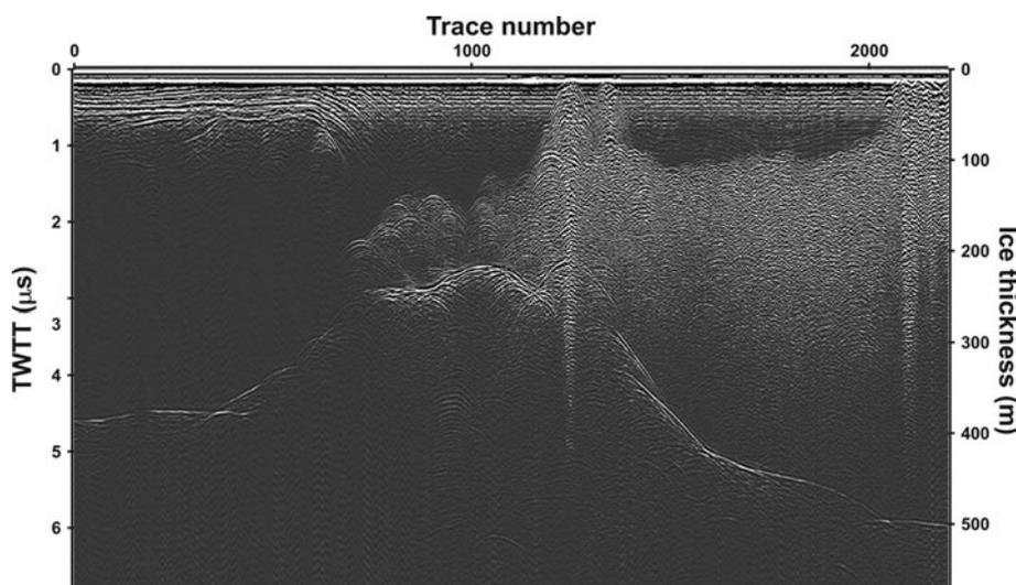
**Fig. 5.** An example of a radar profile recorded using the 20 MHz antennas (Recherchebreen and Hogstebreen, Svalbard, April 2011). The left axis shows the TWTT while the right axis displays the ice thickness, assuming a radio-wave velocity of  $0.168 \text{ m ns}^{-1}$ . Bedrock is clearly visible below 500 m of wet ice.
