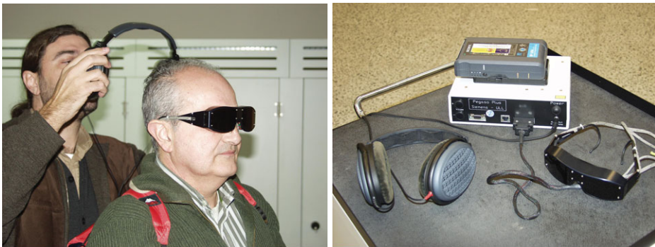
Figure 7. M1 CASBLIP prototype. One-dimensional laser distance sensor provides 64 distances distributed within the horizontal plane at the line of sight level. FPGA based real time adder generates the auditory image.
