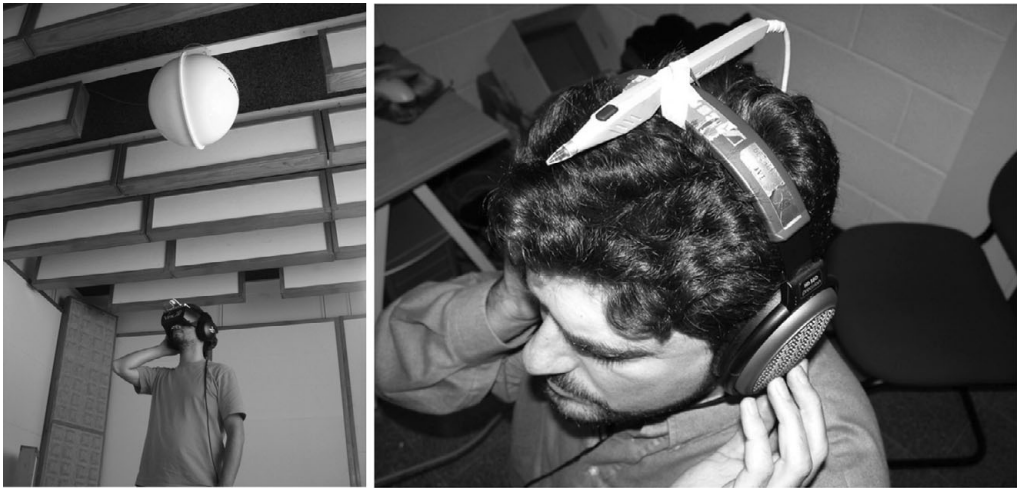
Figure 5. Laboratory system built at ITC, where the user movements are tracked by suitable equipment and a virtual (acoustic) reality is presented accordingly.
