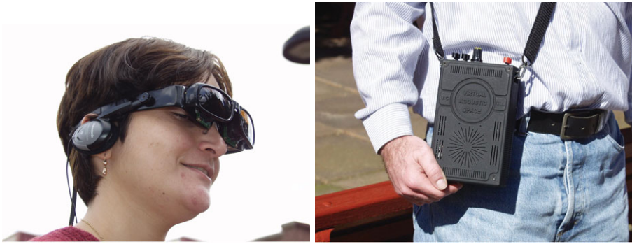
Figure 6. Stereovision based prototype (2002). Based on PC technology, featuring 145 volume elements ( 17 \times 9 \times 8 ).
