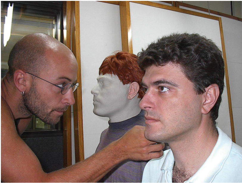
Figure 3. Mannequin built with a very accurate copy of the outer ear, to suppress all practical limits imposed by the user comfort during the HRTF measurement.
