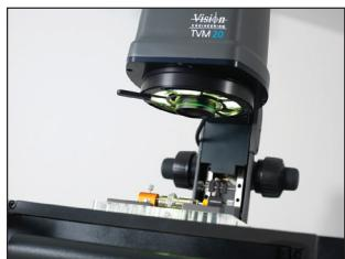
Vision Engineering's TVM Field of View (FOV) video measurement system combines a small footprint with larger system performance and ease of use. Time-saving instant FOV measurements and a moving stage allow larger components to be measured quickly and easily.
