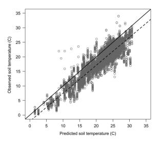
Figure 2. Daily average soil temperature at the 5-cm depth predicted by the soil temperature and moisture model  $(STM^2)$  during the crop rotation and tillage timing experiments relative to observed soil temperature. The solid 1:1 line (y = x) indicates perfect agreement between observed and predicted soil temperature, while the dotted line indicates the fitted regression equation  $(y = 0.96x - 2.1, R^2 = 0.88, P < 0.001)$  between observed and predicted soil temperature.
