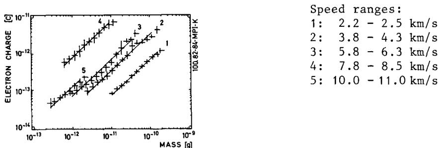
Figure 1. Electron charge versus particle mass. For optical reasons curve 4 shows the charge multiplied by 10. The plotted lines show proportionality.
