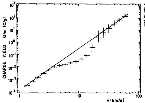
Figure 2. Charge yield  $Q/m$  (ions) plotted against velocity. In the region between 4 km/s and 20 km/s  $Q/m$  shows a deviation from a power law, fitted at low and high velocities.
