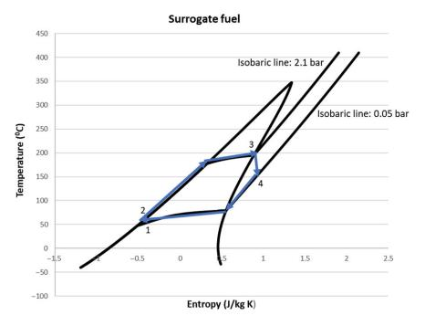
Figure 9. The temperature-entropy diagram of the ORC for the surrogate fuel.
