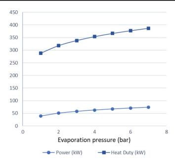
Figure 5. Heat duty and power produced versus evaporation pressure.
