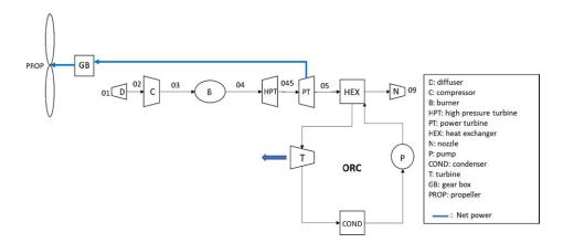
Figure 1. A flow diagram for the whole system.
