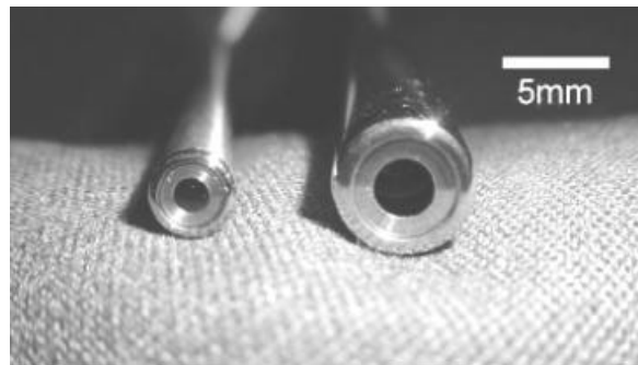
Figure 1: Comparison of the 4.4mm OD confocal arthroscope with the 7mm OD confocal arthroscope
