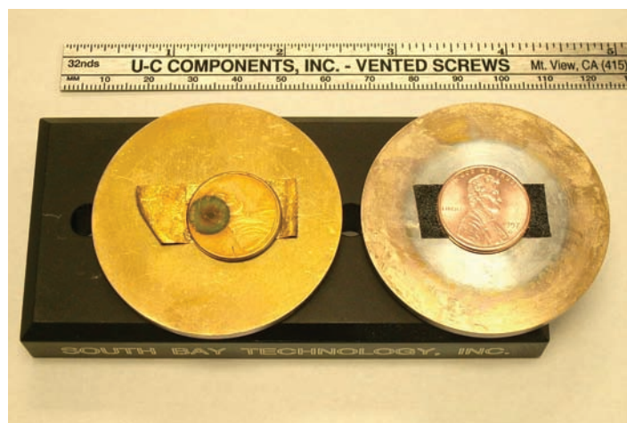
Figure 3 Photograph of two samples Ar ion treated at normal incidence with the standard ion gun (left) and the KDC-10 (right) with after they were heavily coated with gold.
