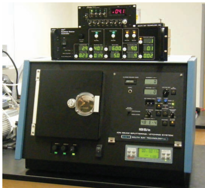
Figure 2 Model IBS/e equipped with the KDC-10 ion source. The ion source power supply is on top and a MKS mass flow controller was used to set up the gas flow conditions for the system.
