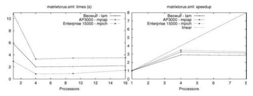
Fig. 10. Runtime and speedup for matrix multiplication. The input is a  $300 \times 300$  matrix of random native integers from 0 to 65535.
