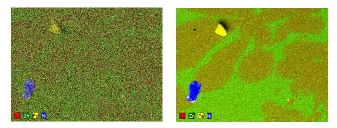
**Figure 2.** EDX Mapping of a duplex brass sample showing  $\alpha$  and  $\beta$  phases with different concentrations of copper and zinc. The left image was obtained with a conventional 10 mm<sup>2</sup> SDD with approximately. 0.01 sr solid angle, the right one with the Rococo 2 detector with a solid angle of more than 1 sr at the same conditions and acquisition time. Images are shown without any post-editing.
