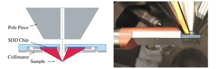
**Figure 1.** Schematic drawing of the Rococo EDX detector positioned below the pole pice (left). A picture of the detector system inside a SEM (right).
