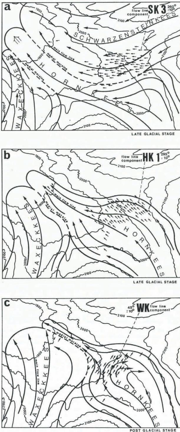
Fig. 16. a-c. Sketches of hypothetical stream lines for former ice movements which were reconstructed from striae, series of crescentic fractures, and crescentic gouges. The small arrows document the ice-flow directions which are constructed from the crescentic fractures and crescentic gouges of 160 stereophotographs. Moraines, the terrain slope, and other morphological details are also considered. a. Schwarzensteinkees; b. Hornkees; c. Waxeckkees.
