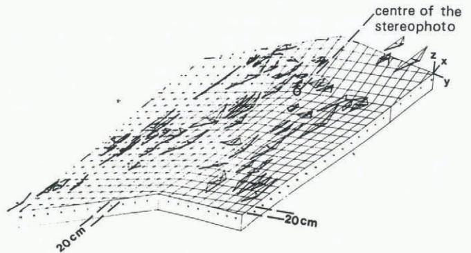
Fig. 14. A "block diagram" made by computer; it is a reduction of the original which had a scale of 1 : 5 (cm). The diagram shows the microforms in three dimensions. With this kind of diagram it was possible to reconstruct the morphological conditions at the test sites.
