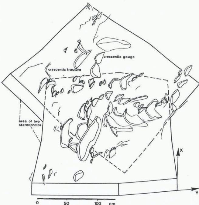
Fig. 12. The interpretation of two pairs of stereophotographs. The crescentic cracks and crescentic gouges are drawn as "isohypses".
