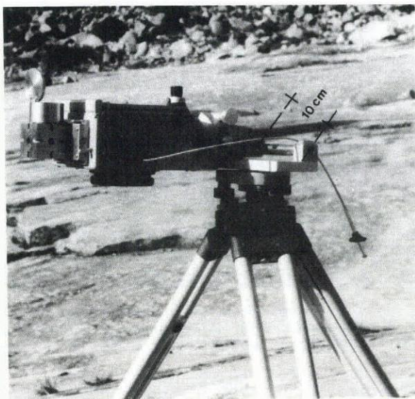
Fig. 8. The Zeiss TMK-6 terrestrial camera with a special carriage; south of the Berliner Hütte.
