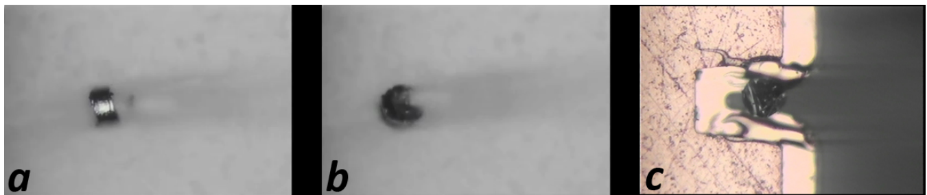
Figure 2. Light optical micrographs of the Pick&Place™ manipulation process for transverse cross section of a 30 μm diameter ceramic fiber. (a) The glass probe approaches a piece of fiber. (b) The glass probe flips the fiber section over and picks it up. (c) The fiber section is positioned onto the EXpressLO™ grid previously painted with glue.
