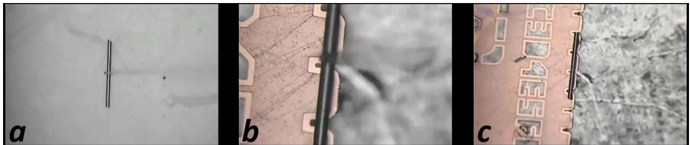
Figure 1. Light optical micrographs of the Pick&Place™ manipulation process for longitudinal cross section of 400 μm long ceramic fiber. (a) The glass probe picks up the fiber. (b,c) The fiber is manipulated onto the EXpressLO™ grid previously painted with glue.
