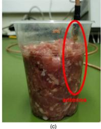
**Figure 13.** (a) Fabricated antenna comparing with one euro cent, (b) complete antenna with coaxial cable and superstrate and (c) antenna embedded into minced pork.
