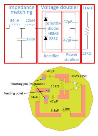
Figure 10. Three-component rectifying system design.
