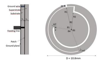
Fig. 1. The circular antenna.
