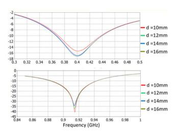
Figure 3. Reflection coefficient of the antenna (at 400 MHz and at 915 MHz).
