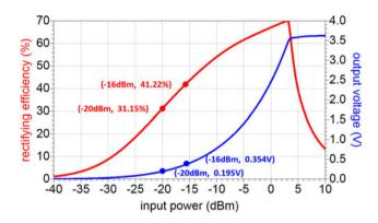
**Figure 8.** Efficiency and output voltage results for different input power (rectifying efficiency = 41.22%, output voltage = 0.354 V with -16 dBm input power; rectifying efficiency = 31.15%, output voltage = 0.195 V with -20 dBm input power).
