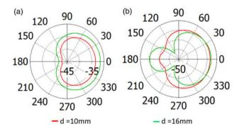
Figure 4. 2D radiation pattern of the antenna at 10 and 16 mm implantation depths ((a) at 400 MHz and (b) at 915 MHz).
