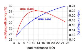
**Figure 9.** Efficiency and output voltage for different load resistances (rectifying efficiency = 31.17%, output voltage = 0.19 V with  $13 k\Omega$  load resistance).
