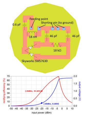
Figure 12. Topology and rectifying results for Skyworks 7630 diode (rectifying efficiency = 35.16%, output voltage = 0.183 V with -20 dBm input power).
