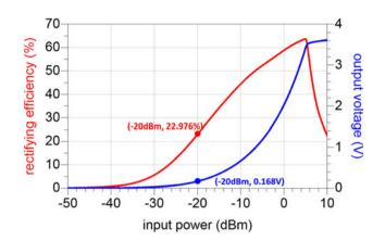
Figure 11. Efficiency and output voltage results for three-component design (rectifying efficiency = 22.976%, output voltage = 0.168 V with -20 dBm input power).
