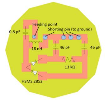
Figure 7. Rectifying system pattern.
