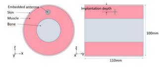
Fig. 2. The three-layer arm model.
