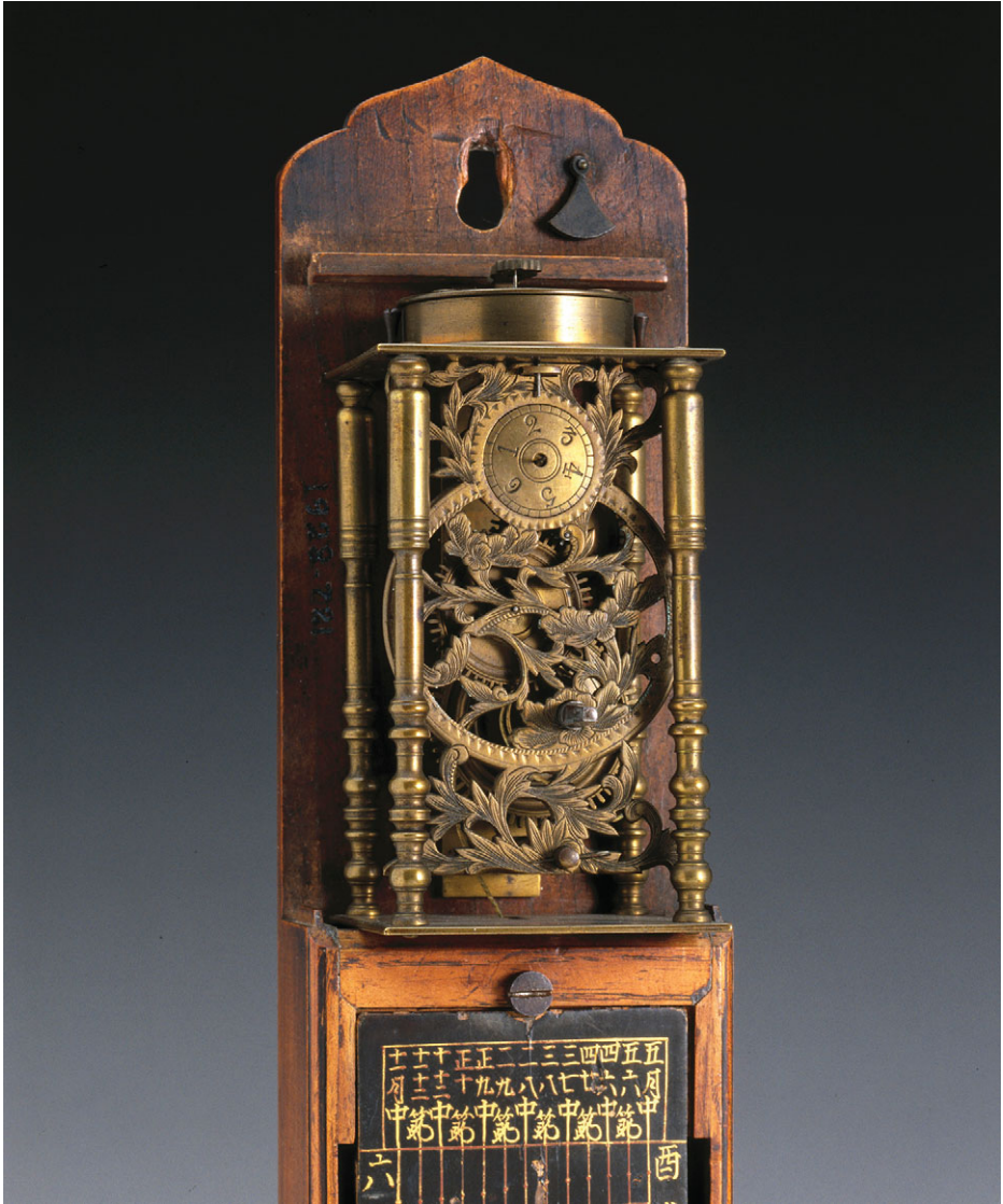
Figure 1.5 Japanese pillar clock, 1800–1870; The “pillar” clock is a type peculiar to Japan, in which the driving weight itself is the time indicator as it falls slowly past a scale of hours mounted below the timekeeping part of the movement. The hour numerals are adjustable by hand to allow for the varying hours of the day and night through the year. The Japanese system of “temporal hours” timekeeping until 1870 divided the day and night each into six equal “hours.” The length of these “hours” differed throughout the year as the seasons changed.
