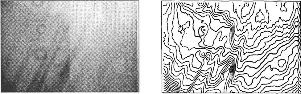
**Figure 2** A MJUO *V* flat field represented *left* as a positive intensity-coded image and *right* in smoothed form as a contour map in which the heavy line represents the mean and the contour spacing is 0.5%. The r.m.s. variation of the flat field is 3.1% with a range of  $\sim 12\%$ . In *U*, *B* and *I* the r.m.s. variations are respectively 3.6%, 3.5% and 2.5%.
