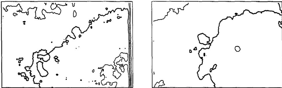
**Figure 4** Contour plots of smoothed  $B$  (sky flat/dome flat) ratios (0.5% contour intervals). *Left* observed ratio, *right* model ratio synthesized from dome flats obtained with full and bisected bandpasses. The plots are very similar.
