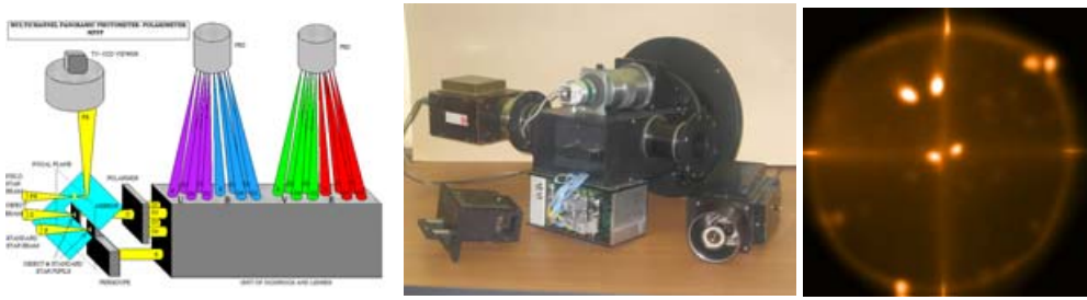
Figure 2. The scheme and the image of multichannel panoramic spectropolarimeter, and the sample star field observed in one-color photopolarimetric mode.
