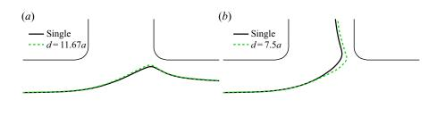
Figure 10. Comparison of the steady trajectory of a capsule train with the trajectory of a single capsule at the same flow split for a/l = 0.6, Ca = 0.1, Re = 10: (a) q = 0.45, d = 11.67a; (b) q = 0.55, d = 7.5a.
