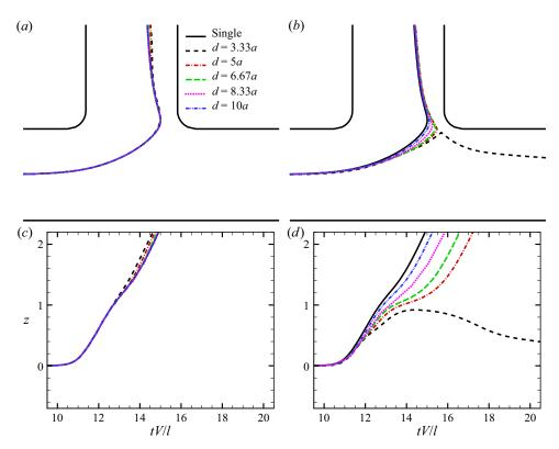
Figure 6. Trajectories of the (a) first and (b) second capsule at the channel bifurcation at different initial interspacing (a/l = 0.6, Ca = 0.1, Re = 10, q = 0.55). The solid lines in (a,b) are the trajectories of a single capsule. Time evolution of the z-axis position of the mass centre of the (c) first and (d) second capsule when it is travelling through the bifurcation region. The solid lines in (c,d) are the results of a single capsule.
