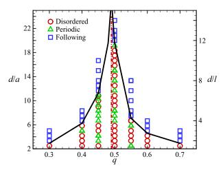
Figure 11. Path-selection states for a capsule train as a function of capsule initial interspacing and flow split ratio for a/l = 0.6, Ca = 0.1, Re = 10. Squares, following; triangles, periodic; and circles, disordered states. Black solid lines, minimum initial interspacing  $d_{ct}$  for following regime; dash-dotted line, critical branch flow ratio  $q_c$  of a single capsule.
