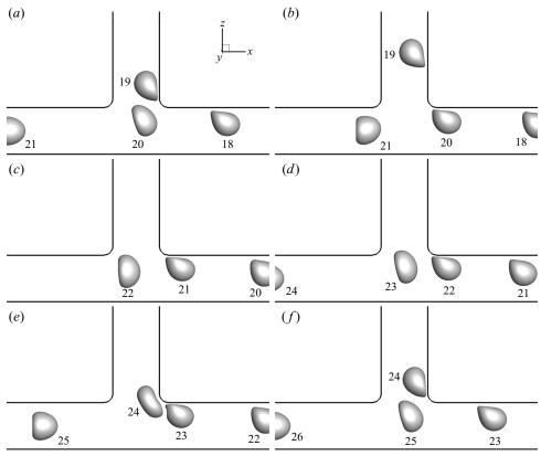
Figure 17. Capsule profiles when the (a) 19th, (b) 20th, (c) 21st, (d) 22nd, (e) 23rd and (f) 24th capsule leaves the channel bifurcation, in the periodic state shown in figure 16. The time instances for (a–f) are 79.2, 81.5, 86.1, 90.2, 95.1 and 97.9, respectively.
