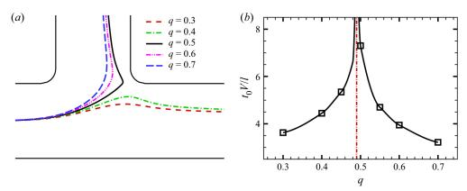
Figure 3. (a) Trajectories of a single capsule at different flow split ratios q. (b) Residence time of the capsule as a function of q. Parameters are a/l = 0.6, Ca = 0.1, Re = 10. Dash-dotted line in (b) marks the critical branch flow split ratio  $q_c$ .
