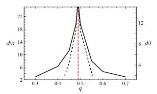
Figure 14. Comparison of the threshold initial interspacings of the two-capsule system and the capsule train (a/l = 0.6, Re = 10 and Ca = 0.1). Black solid line,  $d_{ct}$  for a capsule train; dash line,  $d_{c2}$  for two capsules; dash-dotted line,  $q_c$  of a single capsule.
