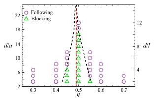
Figure 7. Typical phase diagram of the interaction modes of two capsules for a/l = 0.6, Ca = 0.1, Re = 10. Triangles, blocking mode; circles, following mode; dash–dotted line, critical branch flow ratio  $q_c$  for a single capsule. The dash lines represents the critical interspacing  $d_{c2}$  at which the blocking-to-following transition occurs.
