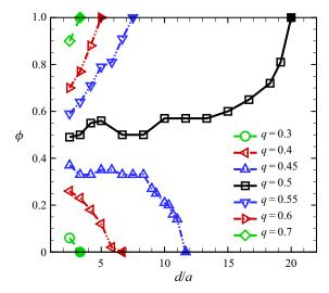
Figure 15. Fraction  $\phi$  of capsules entering the side channel as a function of the initial interspacing d at a/l = 0.6, Ca = 0.1, Re = 10. Full symbols correspond to the steady states; empty symbols correspond to the unsteady states.
