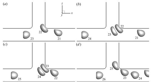
Figure 19. Capsule profiles when the 22nd or 23rd capsule is near the channel bifurcation in the disordered state shown in figure 18. The time instances for (*a*–*d*) are 82.4, 84.2, 87.8 and 92.1, respectively.
