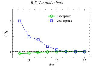
Figure 5. Residence time of the two capsules as a function of initial interspacing d at a/l = 0.6, Ca = 0.1, Re = 10, q = 0.55. The blocking mode takes place at d = 3.33a and the following mode prevails at  $d \ge 5a$ .
