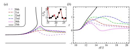
Figure 18. Disordered state: (a) trajectories of individual capsules for a/l = 0.6, Ca = 0.1, Re = 10, q = 0.45, d = 9a, which corresponds to figure 9(c). The figure inset shows the evolution of the capsule residence time  $t_i/t_0$  with respect to capsule index; (b) time evolution of the z-coordinate of the mass centres of capsules in (a).
