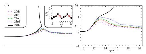
Figure 16. Periodic state: (a) trajectories of individual capsules forming a periodic group for a/l = 0.6, Ca = 0.1, Re = 10, q = 0.45, d = 10.33a, corresponding to figure 9(b). The figure inset shows the evolution of the capsule residence time  $t_i/t_0$  with respect to capsule index; (b) time evolution of the z-coordinate of the mass centres of capsules in (a).
